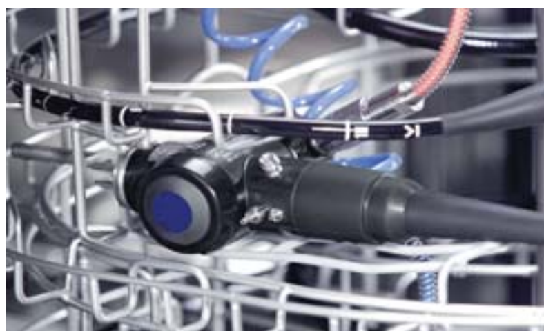
The sophisticated sensor system identifies each individual endoscope and detects leakages
