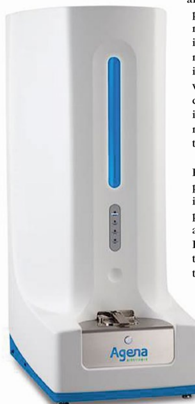
Benchtop MassARRAY mass spectrometry system identify somatic mutations using single base extension with mass distinction of extended primers.
