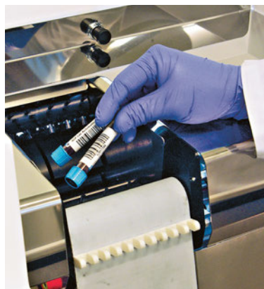
Priority input: Tubes placed here will be processed within seconds
