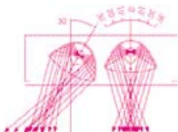
Variable photometric modules enable fully flexible adjustment of the individual lamps
