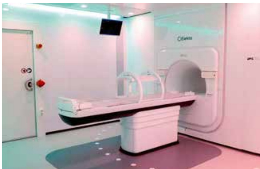
MR-Linac (Unity, Elekta AB, Sweden) at the University of Tübingen (DFG ZI 736/2-1): A hybrid system combining a 1.5-T MRI scanner with a 7-MV linear accelerator for online adaptive MR-guided radiotherapy
