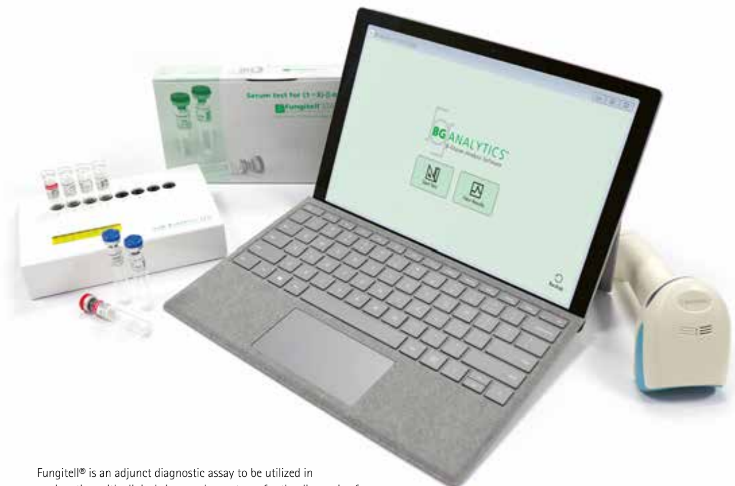
Figure 1: Fungitell STAT PKF08 Instrument The instrument is small in size: 174 mm × 119 mm × 37 mm weighing approximately 1 kg. The power supply is EU friendly. The tablet and barcode reader are presented for size reference.
