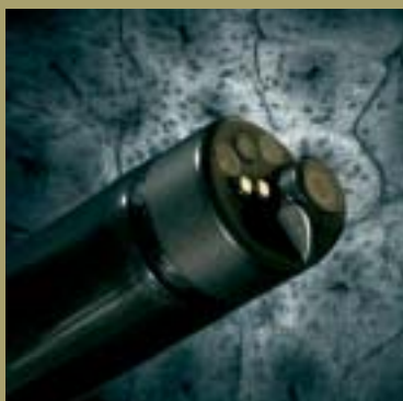
Integrated in the endoscope's distal end, the confocal microscope enables a thousand-fold tissue magnification
