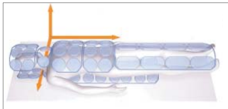
Figure 1: TIM (total imaging matrix) concept. 76 radiofrequency receiver coils in combination with integrated parallel acquisition techniques (iPAT) in all 3 directions allow fast high-resolution imaging of the entire body.
