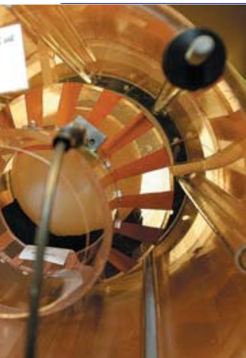
Headcoil - the device in which the head is placed to image the brain
